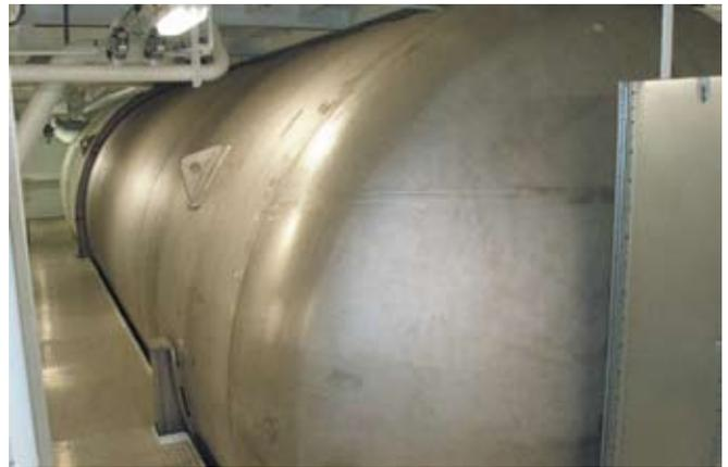
*An LNG bunker tank on a Norwegian cross-fjord ferry*
