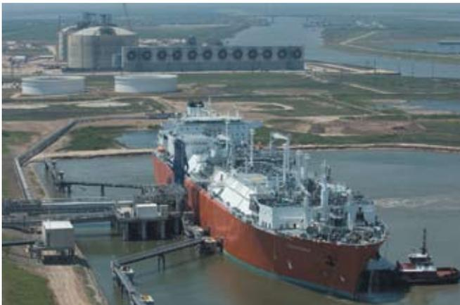
*An operator adapting an LNG receiving terminal for re-exports must consider, amongst a range of issues, the ship's ability to return cargo vapours ashore*
