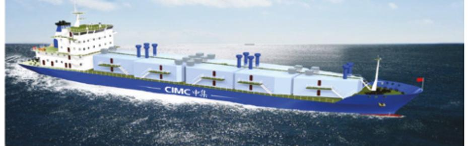
carriage of gases that are liquefied but not compressed natural gas. However, although CNGCs are not addressed in IMO regulations, the philosophy and intent of the IGC Code can be applied to such ships, with appropriate modifications. The same hazards covered in the IGC Code for an LNG carrier, for example, should be considered for a CNGC.
