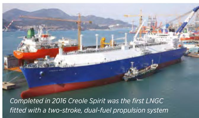
Completed in 2016 *Creole Spirit* was the first LNGC fitted with a two-stroke, dual-fuel propulsion system
