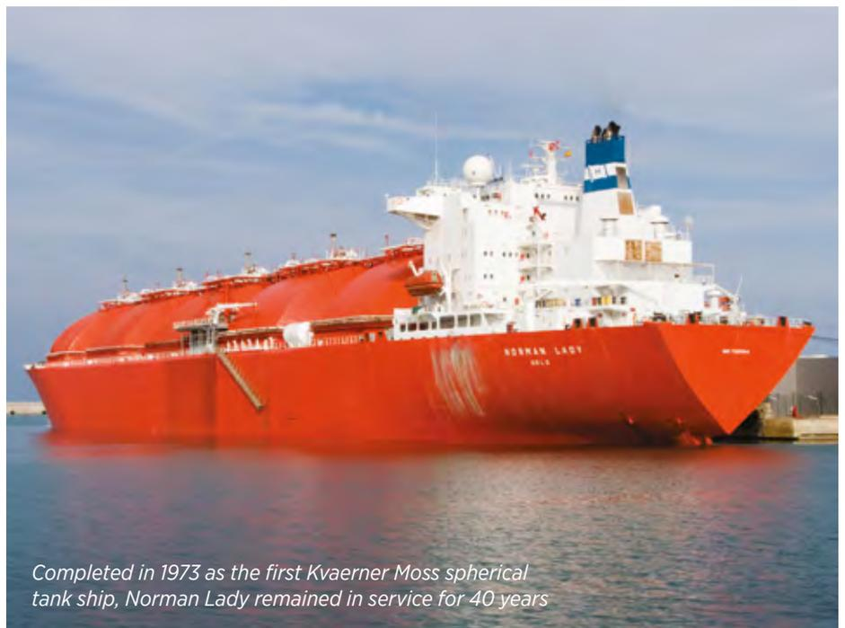
Completed in 1973 as the first Kvaerner Moss spherical tank ship, Norman Lady remained in service for 40 years
