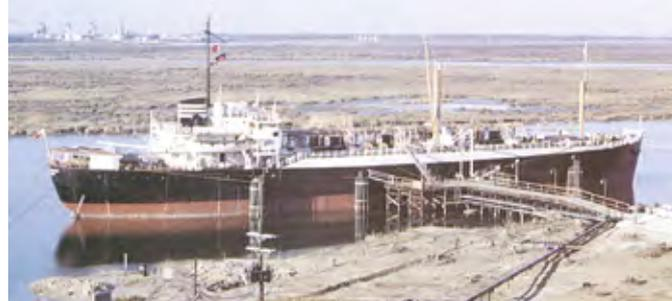
The 931 m<sup>3</sup> *Descartes*, built for Gazocéan by La Ciotat, was the first semi-pressurised/semi-refrigerated (semi-ref) LPG carrier
