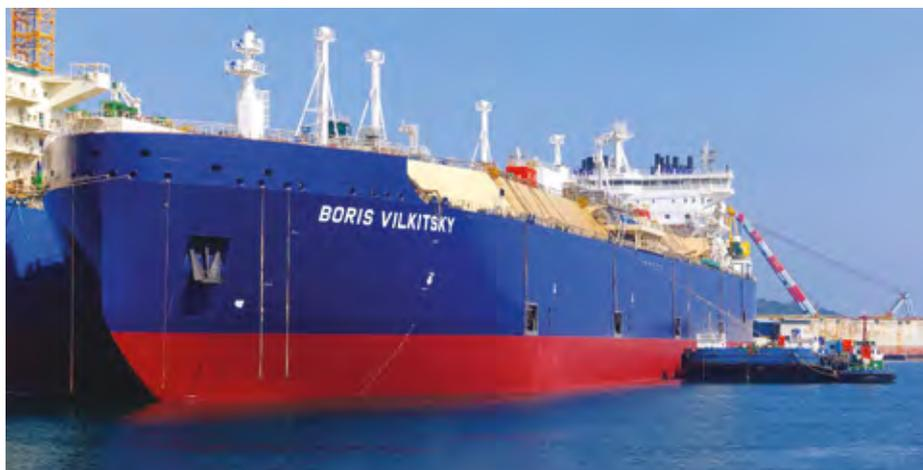
*Boris Vilkitsky is one of five 172,000 m<sup>3</sup> icebreaking LNG carriers operated by Dynagas in the service of the Yamal LNG project*
