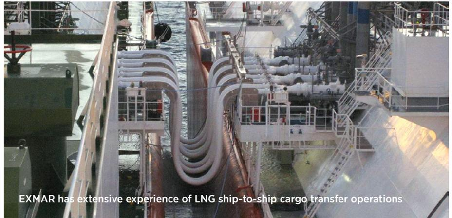
EXMAR has extensive experience of LNG ship-to-ship cargo transfer operations
