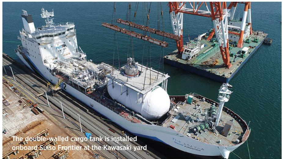
The double-walled cargo tank is installed onboard *Suiso Frontier* at the Kawasaki yard
