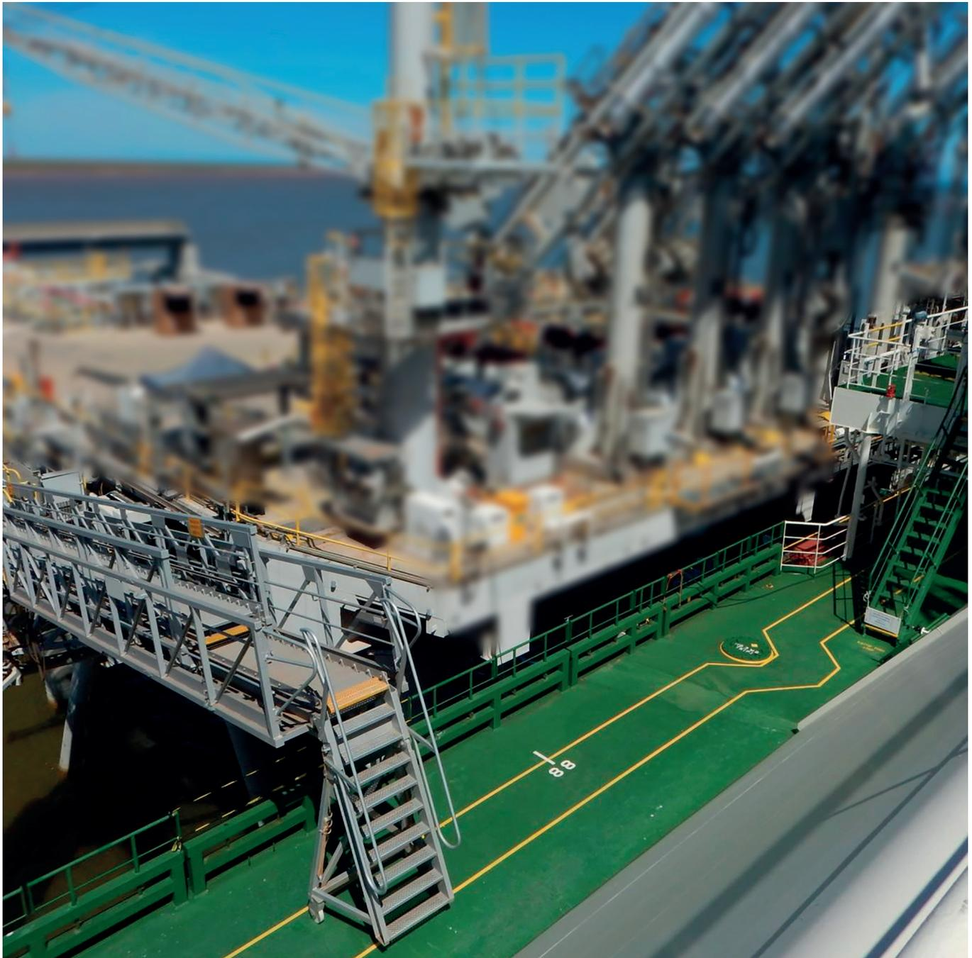
Figure 10: Transverse exit deck ladder
