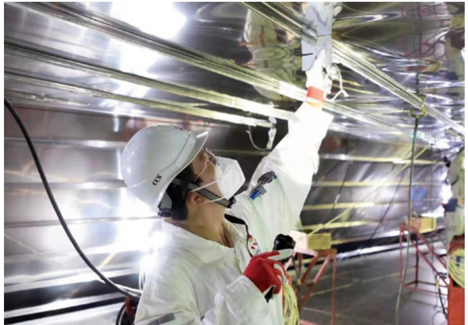
A CCS surveyor verifies the integrity of an LNG carrier newbuilding's GTT NO 96 membrane containment system
